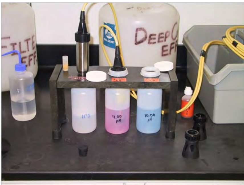
Left: Probe calibration stand with rubber stopper feet.
