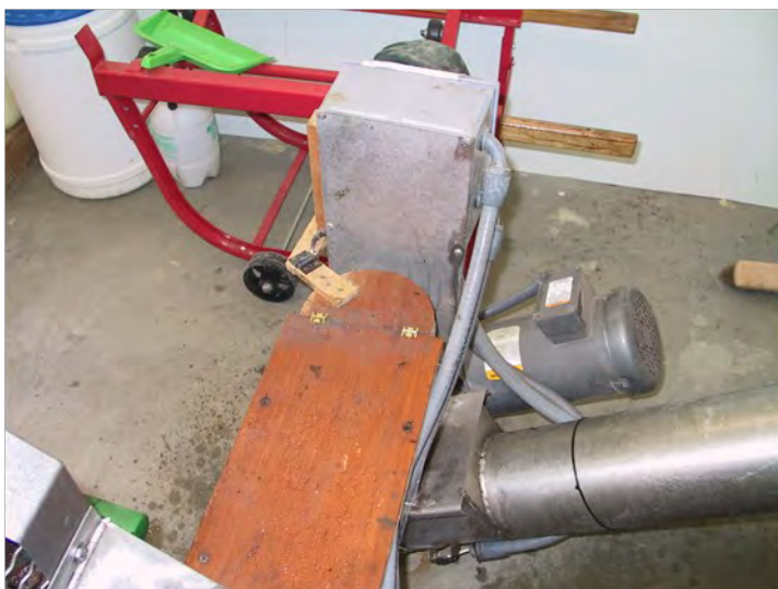
Left: Mods that Roger did to shut down the press in case cake accumulated in the auger junction.
