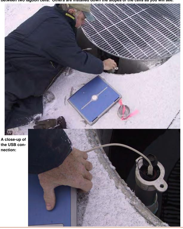
Chuck has the depth data loggers configured to read the lagoon cell depth once per day. In the shot below of his laptop screen, he's retrieved the accumulated data from 12/6 to 12/27/2011. The columns displayed (in order) are the date, Feet of depth, battery voltage, and something called "pulses" (I'm not familiar with that last one). From his laptop, Chuck can delete the old data on the transducer if needed, save it to a file, reconfigure the datalogger parameters, etc.
