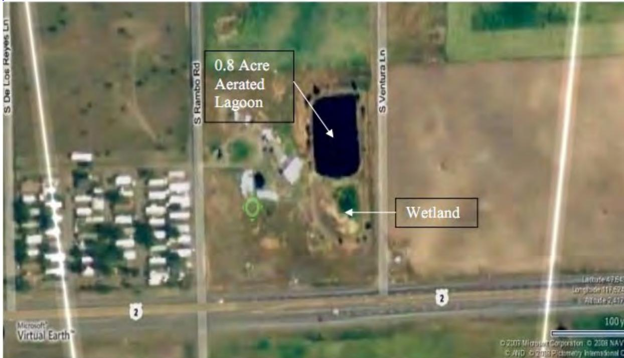
This is a STEP (septic tank effluent pumping) system with aerated lagoon discharging to a small wetland.
