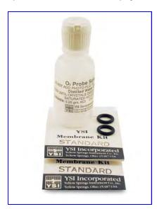
at \$8.50 and change. Salvaging the used cap, and replacing just the membrane, it's only \$1.07 a pop.
